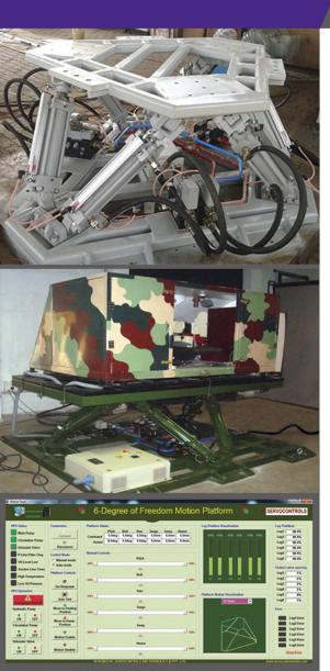
**Summary:** A standard way of building motion simulators is to start with a Stewart platform. Stewart platforms enable movement with six degrees of freedom (x, y, z axis transitions, plus pitch, yaw and roll rotations).
